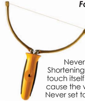
Never shorten the cutting wire to less than 5.5" from post to post. Shortening or bending the wire far enough around to touch itself will overheat and ruin your unit and will cause the wire to become extremely hot. Never set tools on metal while turned on.
